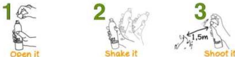
BoldFoam F-40 acts upon hot vegetal oil **saponifying** the grease and converting it into soap which is easily removable with water. The application by light foam makes it that soft for not to start dangerous splashes during the extinction that may even propagate the fire out of the initial boundaries.
